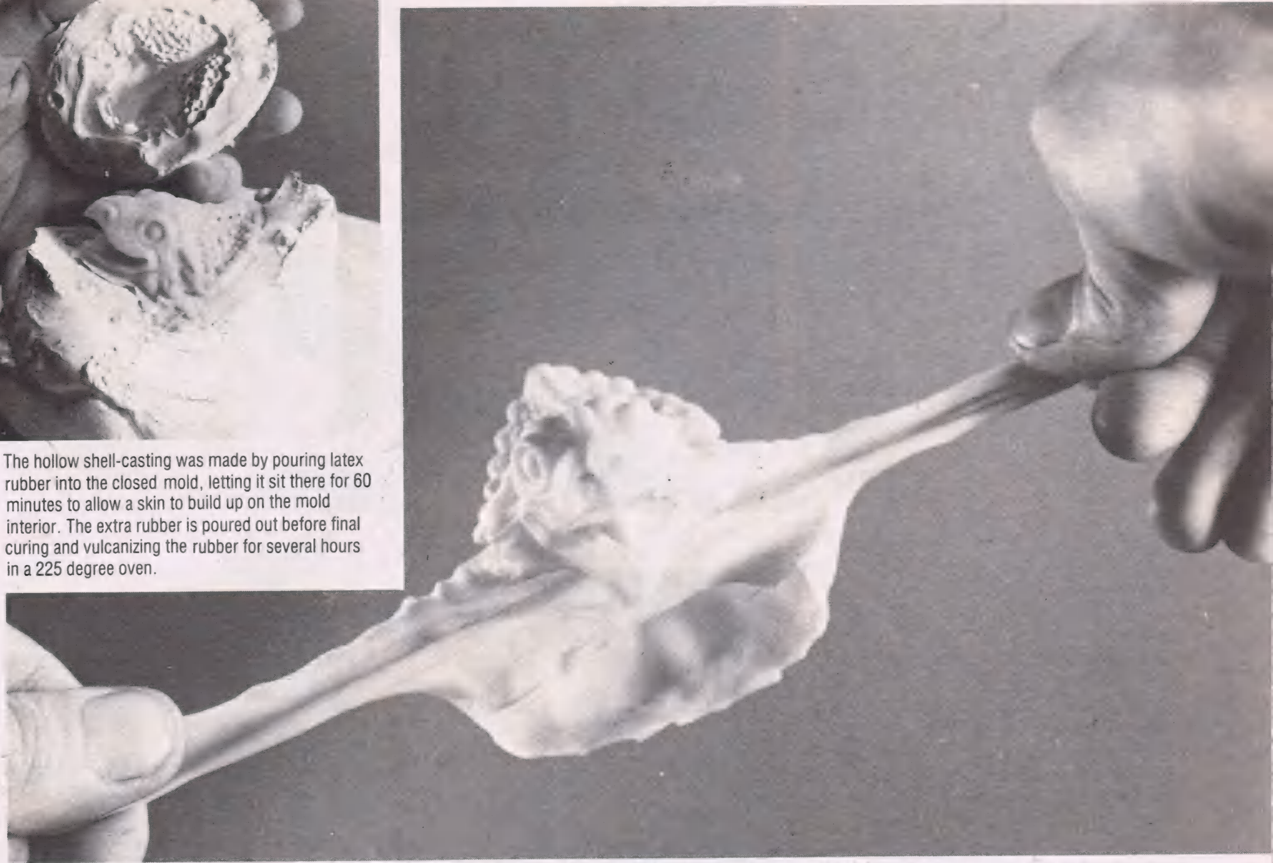
The third section of the mold has been completed and the first latex "shell casting" or slush casting has been completed.
